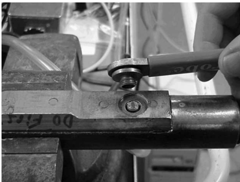
FIG. A1.1 Membrane Wrench Shown with Membrane Removed Exposing the Sub-Membrane Fittings
